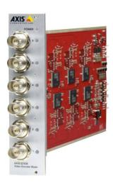
AXIS Q7436 Video Encoder Blade is a 6-channel encoder blade with support for 60/50 fps.
